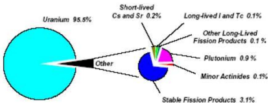
Figure 6. Composition of Spent Nuclear Fuel (standard PWR 33 GW/t, after 10 years of cooling)<sup>9</sup>
