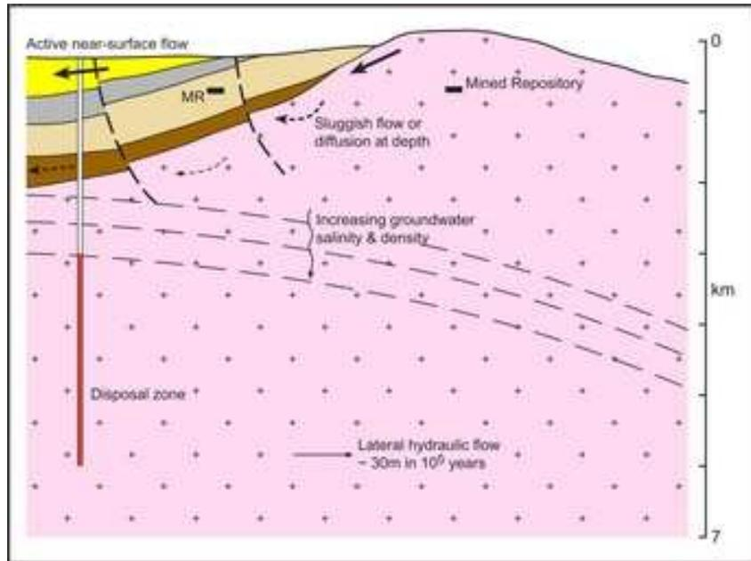
**Figure 13. Deep Borehole Disposal Concept<sup>46</sup>**
