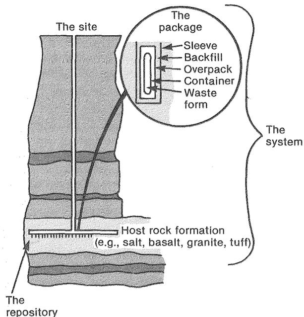
Mined geologic disposal will use a system comprised of engineered barriers (the waste package and the mined repository) and naturally occurring barriers (the host rock formation and the chemical and physical properties of the repository site itself) to provide long-term isolation of waste from the biosphere.
