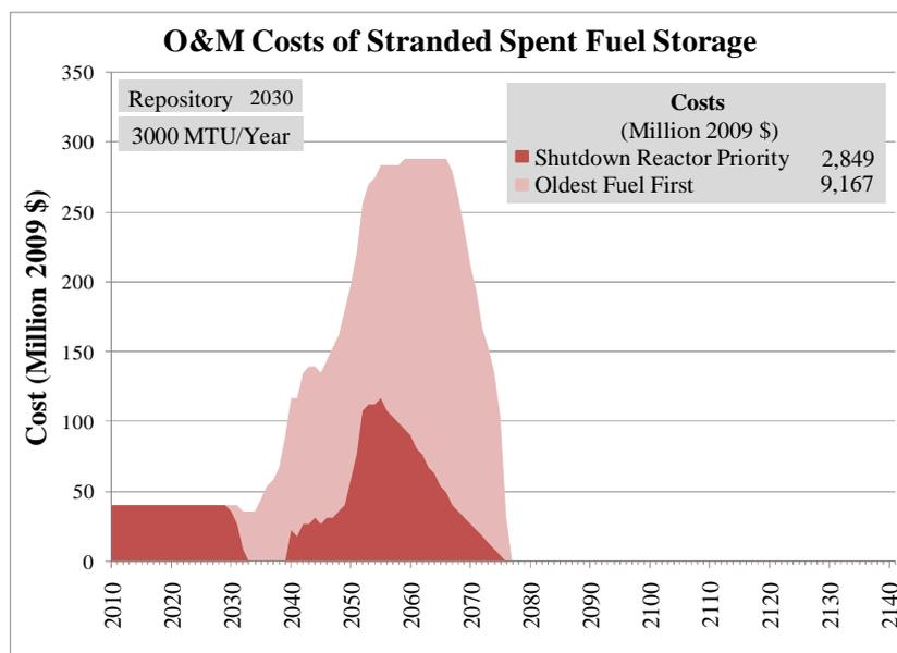
**Figure 16. Operation and Maintenance Costs of Stranded Spent Fuel Storage**<sup>71,72,73</sup>
