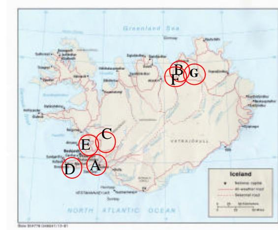
Figure 26: Location of Hellisheidi [A, 213 MW], Krafla [B, 60 MW], Nesjavellir [C, 120 MW], Reykjanes [D, 100 MW], Svartsengi [E, 76 MW], Bjarnafلاغ [F, 3 MW] and Husavik [G, 2 MW].
