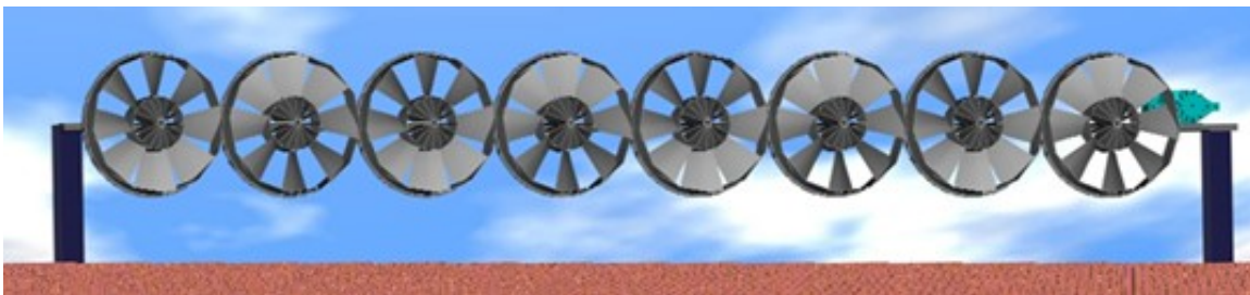
Figure 14. Battery of eight microturbines to be placed on a building roof.
