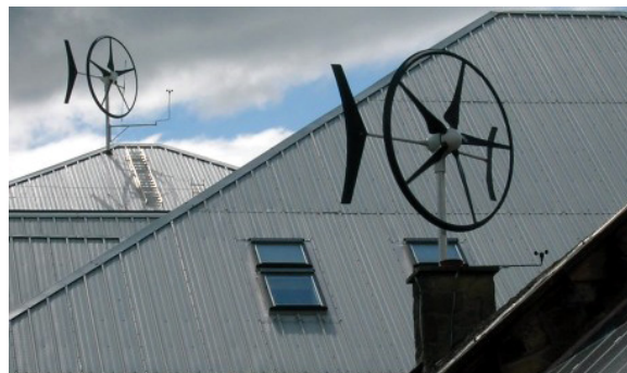
Figure 5. Inoperational small Bergey 1500 wind turbine on top of university building at Melbourne Australia, 2000. Photograph: Paul Gipe.
