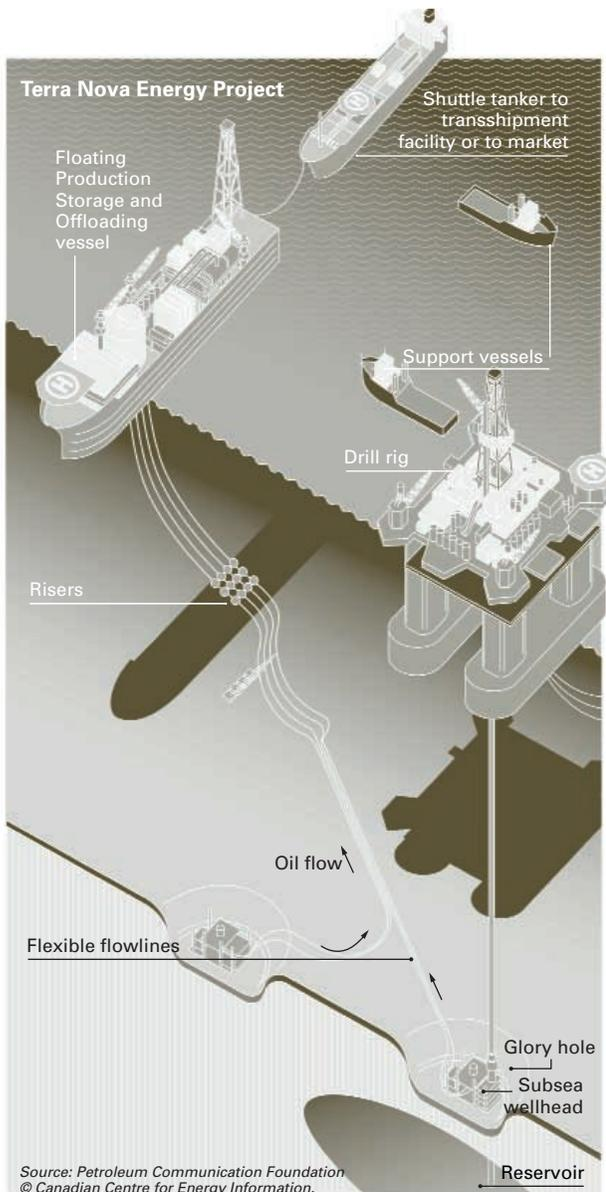
more than 40 kilometres of flexible flowline is used to convey hydrocarbons to and from the wells. Produced gases are separated from the oil and re-injected into the reservoir for possible future extraction.
