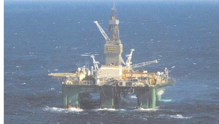
Eirik Raude, a semi-submersible drilling vessel that drilled an exploration well in very deep water offshore Nova Scotia in 2003. The Eirik Raude and its sister ship are the largest semi-submersible vessels in the world.
