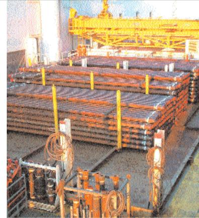
Various types of marine riser and drilling pipe are stocked aboard an offshore platform.
