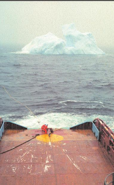
As part of Hibernia's ice management strategy, encroaching icebergs are "lassoed" with a heavy cable and towed by a support vessel into a different trajectory.
