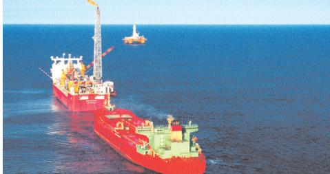
The Terra Nova floating, production, storage and offloading vessel.
