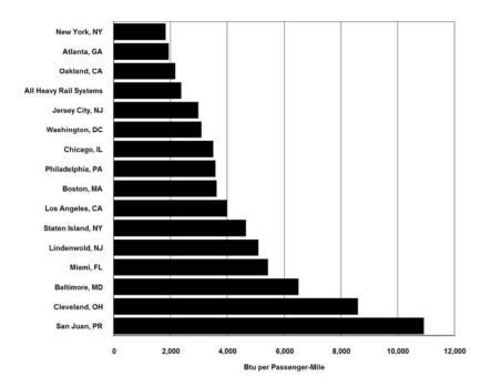
Figure 2.3. Energy Intensity of Heavy Rail Systems, 2009
