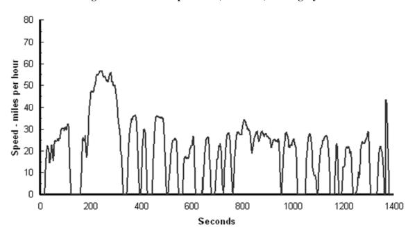
Figure 4.6. Cold Temperature (Cold FTP) Driving Cycle
