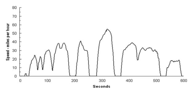
Figure 4.5. Air Conditioning (SC03) Driving Cycle
