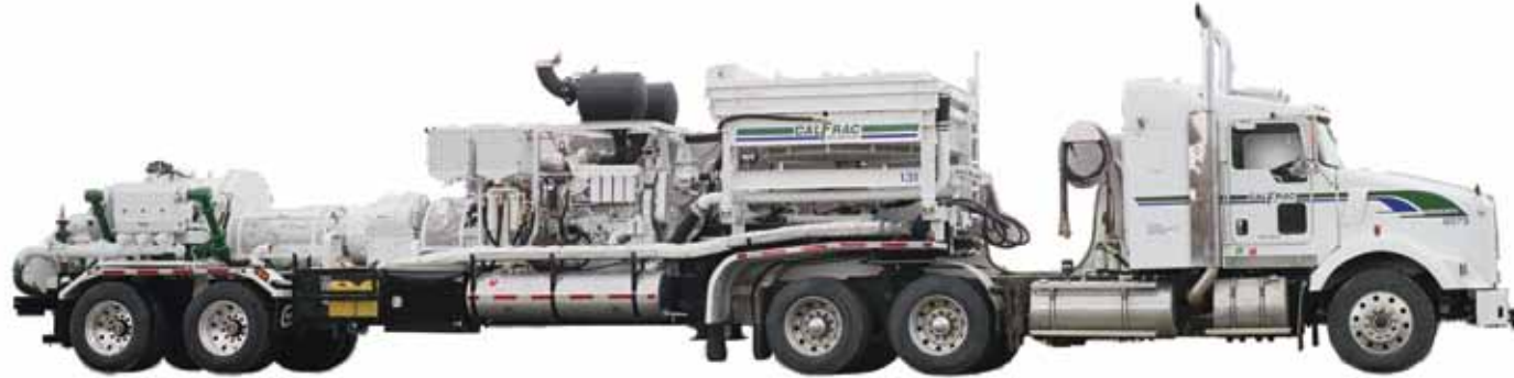
Frac Pumping Unit
