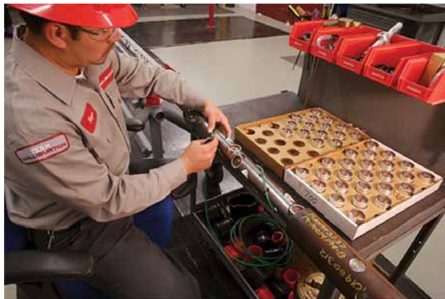
Preparation of perforating tool
