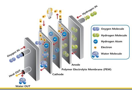
Fuel cells directly convert the chemical energy in hydrogen to electricity, with pure water and potentially useful heat as the only byproducts. Hydrogen-powered fuel cells are not only pollution-free, but also can have more than two times the efficiency of traditional combustion technologies.
