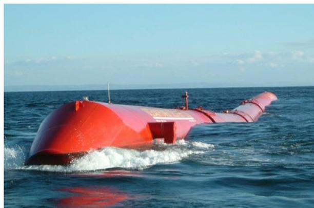
deployed in a Danish inlet in 2003 (Fig. 14.14). Activities are under way for installation of full-scale devices in Denmark (1.5 MW in 2011) and Wales (7 MW in 2012). Wave Energy AS has plans for a 300 kW multi-reservoir, shoreline device in Denmark during 2011;
