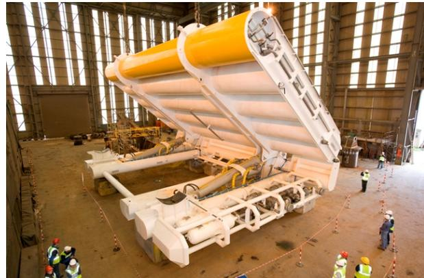
length of the structure, it raises and lowers the independent floats, each driving a hydraulic pump that is connected to a common hydraulic motor and generator. A 1/10th scale system has been running in Denmark since 2006 and the first section of the 500 kW device was installed in September 2009.
