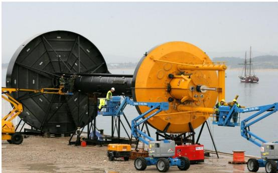
**Figure 14.7** CETO Float and Pump Unit prior to deployment (Source: Carnegie Wave Energy)
